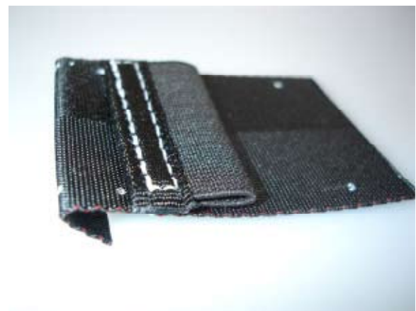
2.5 Stitch Elastic Keeper onto TYPE 12 Webbing as shown. Use Nylon E Thread
