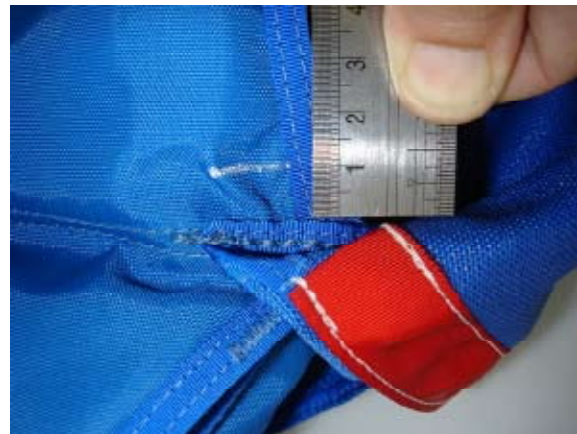
4.9 Mark 10mm along Flap #1 from intersection as shown
