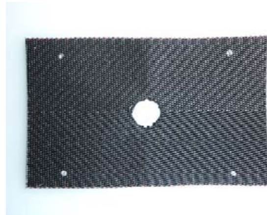
2.4 Cut TYPE 12 Webbing as per Template
