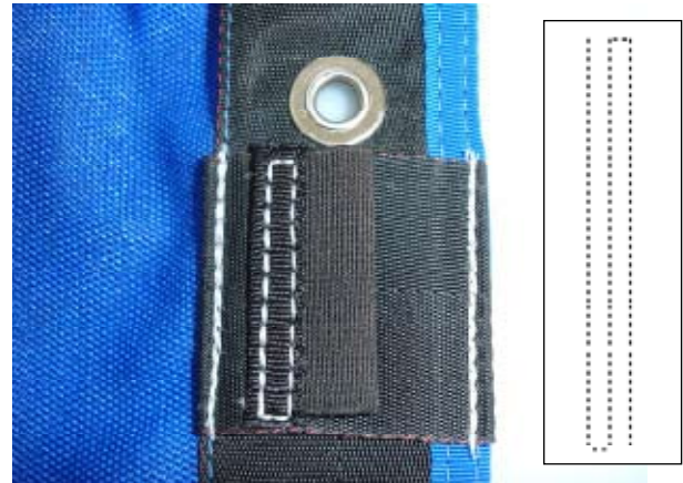
3.2 Fold edge of TYPE 12 webbing and stitch opposite side down on top of Edgebinding
